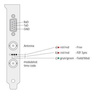
The coaxial antenna connector, two status LEDs and a 9 pin sub D connector can be found in the rear slot cover. (see figure).
