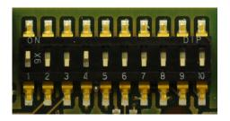
Pin 1: DIL 1 or DIL 8 ON Pin 4: DIL 5 or DIL 10 ON Pin 7: DIL 3 or DIL 7 ON
